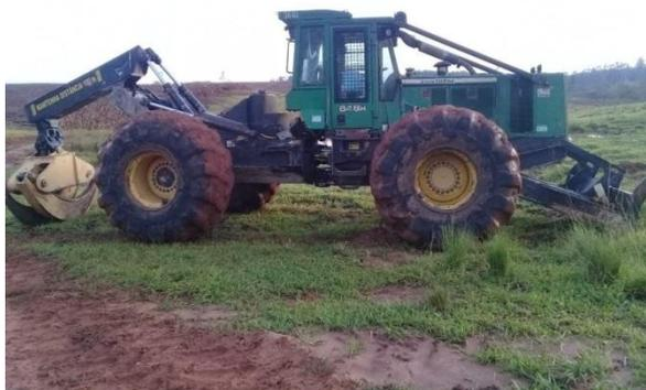
Figura 1: *grapple skidder* marca *John Deere* – modelo 848 H.
